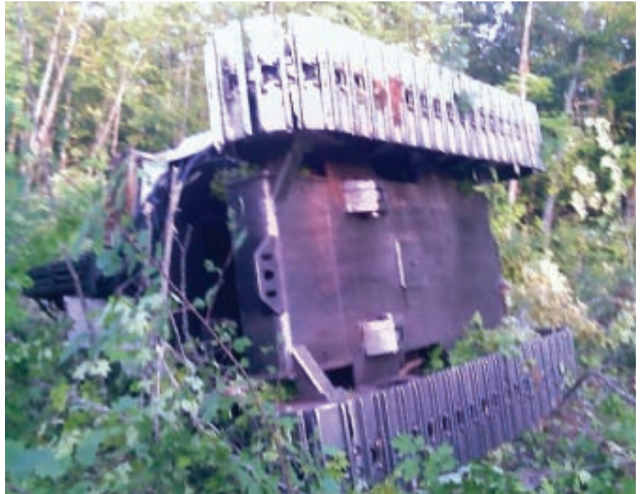
The feller-buncher tipped after running up on a stump while in a hardwood stand.
